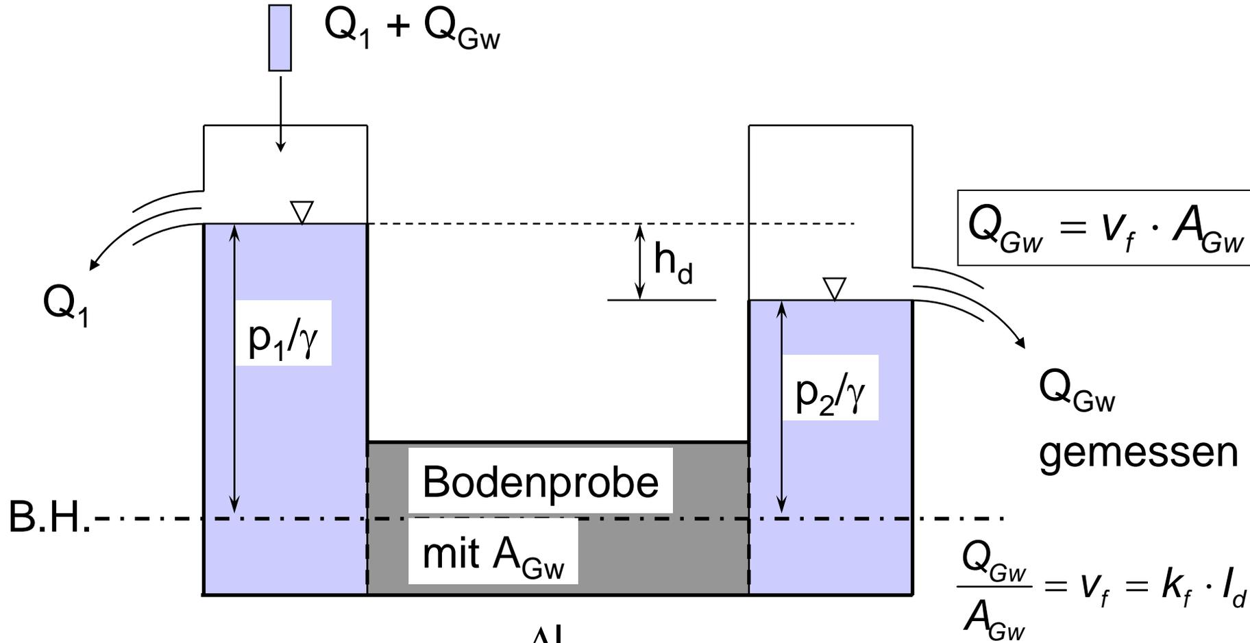
$$\frac{p_1}{\gamma} = \frac{p_2}{\gamma} + h_d \quad h_d = \frac{p_1}{\gamma} - \frac{p_2}{\gamma} \quad l_d = \frac{h_d}{\Delta l}$$
